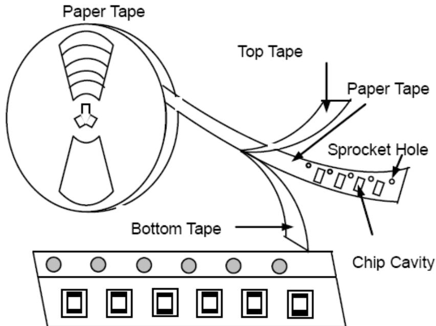
**Remark:** The sprocket holes are to the right as the tape is pulled toward the user.
